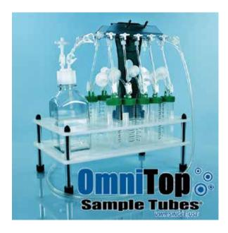
connected to the bioreactor with a commonly used tube welder. After connecting a syringe to the 0.2µm filter, air can be driven into the OmniTop which forces fluid into the bioreactor via the dip tube. Because OmniTop is a closed system it has greatly simplified any small volume addition to a bioreactor and is now being used for many upstream Bioprocess applications.
